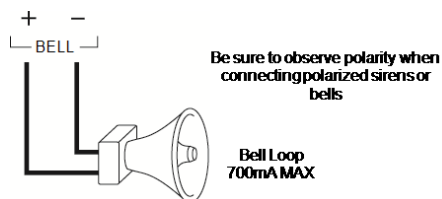
Figure 2-13 Bell Wiring
